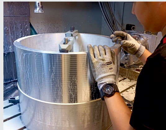
GreenMotor cooling tube milling
